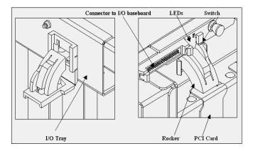
Figure 3-9: Rocker Mechanism
